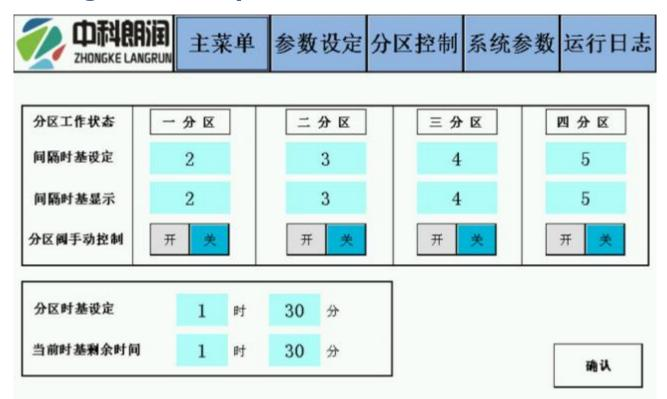
The following figure shows the partition control interface. This interface is used to set different lubrication cycles for different partitions in the partition mode to meet the automatic control in the complex partition mode.
